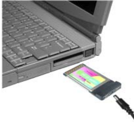
Fig 5-1 Install the CardBus adapter and switching power adapter
