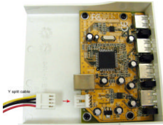
Figure 6-2 Connect Y split cable to USB 2.0 4-Port Bay Hub
