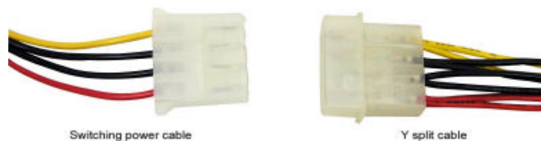
Figure 6-1 Connect Y split cable to switching power cable
