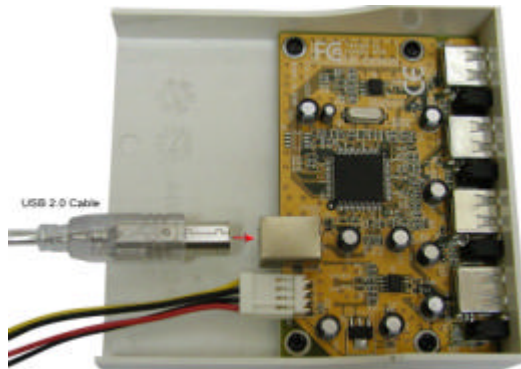
Figure 6-3 Connect type B plug to USB 2.0 4-Port Bay Hub
