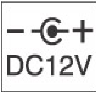
Polarity of DC plug
