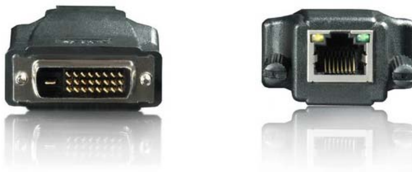
Figure DVI over CAT5e Mini-Extender layout
