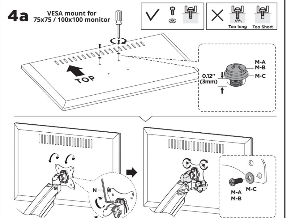
**IMPORTANT NOTE:** Ensure the four bolts for the rotation on the VESA head are tightened first before installing your monitor. Not doing so may result in the VESA head and your monitor detaching.
